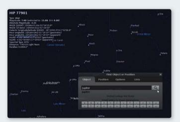
Try searching for something that isn't currently visible. Select the fourth icon in the left toolbar to open the Search window. On the Object tab enter the name of an object, then click the magnifying glass. The display will rotate until the object is centred.
